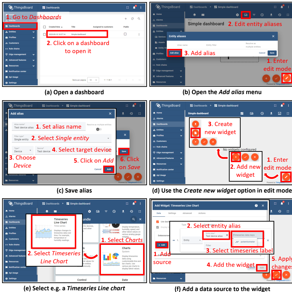
Figure 10: Steps to create and edit a simple dashboard, including a chart widget recording telemetry from an existing device as data source.
